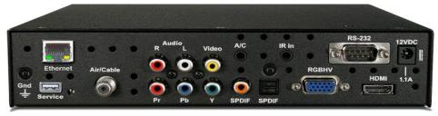
The new 232-ATSC 4 HDTV Tuner, our 4th-generation ATSC HDTV tuner, adds new capabilities to the industry-standard 232-ATSC series. New features include tuning MPEG-4 programs, up to 1080p output, and more efficient operation. The new tuner is fully compatible with control commands for previous models.
