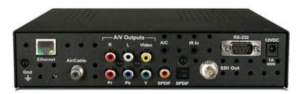
Ethernet and Web page: RJ-45 10/100 Ethernet connector
