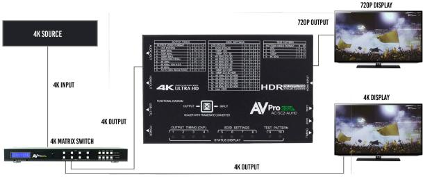
WITH THE AC-SC2-AUHD YOU ARE ABLE TO DOWNSCALE (AS SHOWN) OR UPSCALE A SIGNAL TO DISTRIBUTE THE BEST POSSIBLE PICTURE TO ANY DISPLAY.
