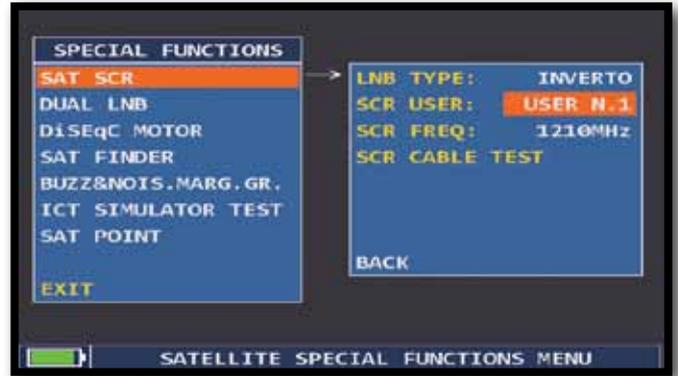
NAVIGATE IN "LNB TYPE" AND CHOOSE THE LNB/MULTISWITCH MODEL,
