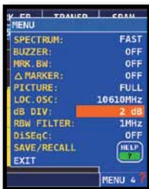
NAVIGATE IN “MENU&?” FROM THE SAT SPECTRUM SCREEN, SELECT “DB DIV 2DB” AND “RBW FILTER 1 MHz”.
