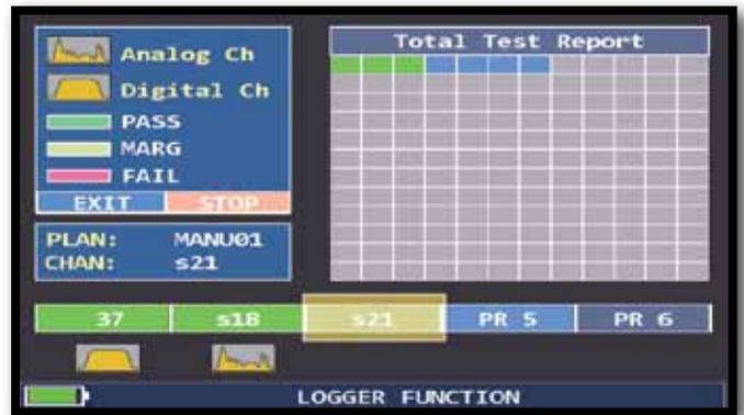
NAVIGATE IN “SAVE DATALOGGER” AND SET THE PARAMETERS REQUIRED. TOUCH “START SAVE” TO CREATE A NEW LOG FILE
