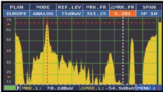
C/N MEASUREMENT MODE "IN BAND" THE SIGNAL/NOISE RATIO IS MEASURED BETWEEN THE SIGNAL LEVEL OF THE VIDEO CARRIER (SIGNAL/CARRIER, RED MARKER) AND THE NOISE LEVEL, ESTIMATED IN THE BAND BETWEEN THE COLORED SUBCARRIER AND THE AUDIO CARRIER (WHITE MARKER),
