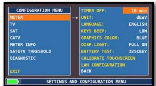
NAVIGATE IN “CONFIGURATION MENU” THEN “METER” IN THE VOLUME SCREEN AND SET THE “TIMER OFF” VALUE REQUIRED. THE METER WILL TURN OFF AFTER 5 OR 10 MINUTES OF INACTIVITY. PRESS ANY KEY TO INTERRUPT THE AUTOMATIC TURN-OFF.
