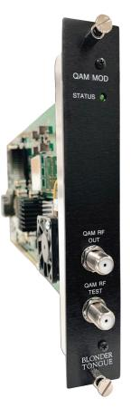
The NXG-32CH-QM (QAM Output Module) is part of the Blonder Tongue NeXgen Gateway (NXG) platform. The NXG-32CH-QM multi-channel QAM modulator provides up to 32 QAM 256 channels. All 32 output channels are fully agile from 54 to 1002 MHz, with the requirement that all channels must be within a 768 MHz frequency span. Each program can be configured to support a customized channel lineup for desired locations.
