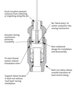
Corning Gilbert introduces the next generation in 2piece connector technology, with patented design features that provide clear performance advantages over traditional two piece connectors.
