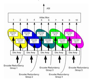
1:1 Encoder Redundancy Connections-Graphic
