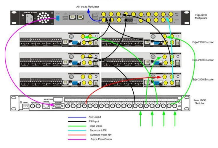
N + 2 Encoder Redundancy- Illustration
