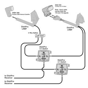
DISH 500 with DishPro Twin LNBF, DISH 300 with a Single LNBF, Two DP21 Switches, and a DishPro Compliant Splitter. Supports two receivers from three satellite locations.
