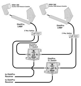
Two DISH 300s with Single DishPro LNBFs, Two DP21 Switches, and Two DishPro Compliant Splitters. Supports two receivers from two satellite locations.
