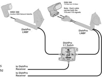
One Dish 500 with a Twin LNBF, One Dish 300 with a Single LNBF, and One DP21 Switch. Supports one receiver from three satellite locations and one receiver from two satellite locations.
