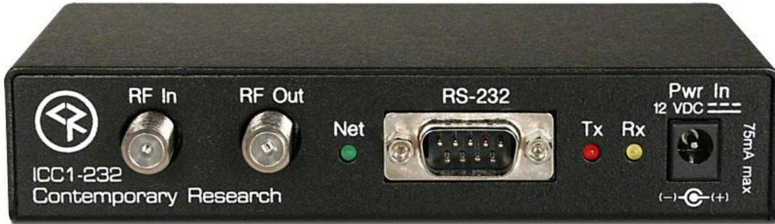
The ICC1-232 RS-232 Display Controller delivers economical 1-way control for power, volume, channels, and available control lockout commands, receiving iCC-Net network commands over the same broadband coax that carries the CATV channels. Compact in size and price, the ICC1-232 features discrete power control and intelligent tuning from a channel list stored in onboard non-volatile memory. Tuning options include analog- and HDTV-format channels.
