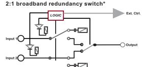
\*4 x 2:1 broadband redundancy-switch boards integrated into unit
