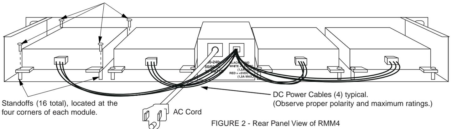
FIGURE 2 - Rear Panel View of RMM4
