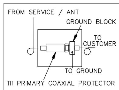
COAX CABLE FROM SERVICE PROVIDER OR ANTENNA
