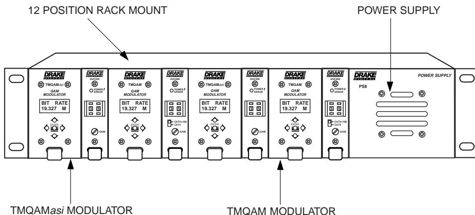
The R.L. Drake model TMQAM and TMQAMasi modulators are professional quality modular digital headend components designed to provide optimum performance with minimized rack space requirements. These modulators accept an MPEG2 transport stream input in either the SPI format or ASI serial format, depending on the model, and is capable of providing a QAM output with 16, 32, 64, 128, or 256 constellation points.
