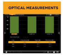
Once the optical fibre input enabled, and thanks to the optical receiver (whether selective or not), optical attenuation measuring can proceed for three wavelengths (1310 nm, 1490 nm, and 1550nm) and their powers, as does RFoG installation analysis.
