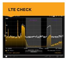
It analyses the impact of the LTE signal on the DTT channels, and detects whether the use of filters is required. Furthermore, it allows spectrum simulation upon the introduction of the LTE filter recommended by the meter itself. A list of filters is displayed for the user to choose the one that best fits his/her requirements.
