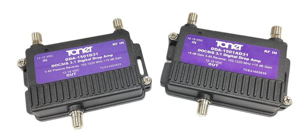
The Toner DDA D31 Series Digital Drop Amplifiers are the latest addition to the Toner range of DOCSIS 3.1 compatible products. These drop amplifiers have a frequency range of 5 to 1220 MHz with a reverse or upstream bandwidth of 5-85 MHz. Two models are available, one with passive reverse and one with 8 dB gain in reverse.
