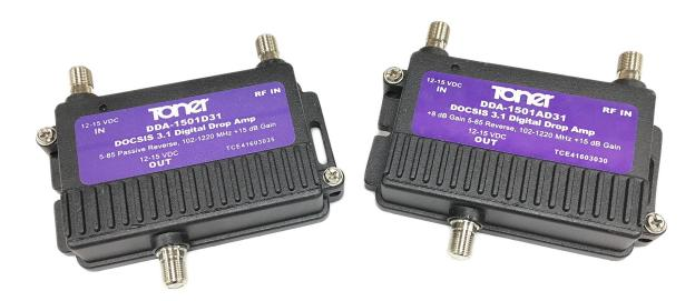
The Toner DDA D31 Series Digital Drop Amplifiers are the latest addition to the Toner range of DOCSIS 3.1 compatible products. These drop amplifiers have a frequency range of 5 to 1220 MHz with a reverse or upstream bandwidth of 5-85 MHz. Two models are available, one with passive reverse and one with 8 dB gain in reverse.
