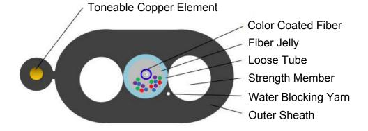
The FDC Series Flat Drop Cable from Toner is an industry standard Loose Tube fiber drop cable for FTTP applications. This flat drop cable is available with 1, 2, 6 or 12 count fiber with a toneable copper component embedded in the polyethylene jacket.
