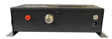
The HDDM from Toner is an economical encoder/modulator that is ideal for places such as bars, restaurants, schools or anywhere that a digital TV channel needs to be added to the existing cable system. The small form factor allows mounting on a wall panel or on a rack shelf. With an HDMI input, the HDDM allows easy encoding and modulation to an RF output from 47-999 MHz. Setup is easily accomplished via the front controls or by a GUI and IP interface.
