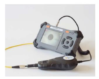
The quality and cleanliness of a fiber optic connector is imperative to a quality optical connection. Connectors with dust, scratches, chips or a poor polish, even when new can drastically affect the system performance in a fiber optic link. For these reasons, it is important to inspect the end face of the fiber in the connector.
