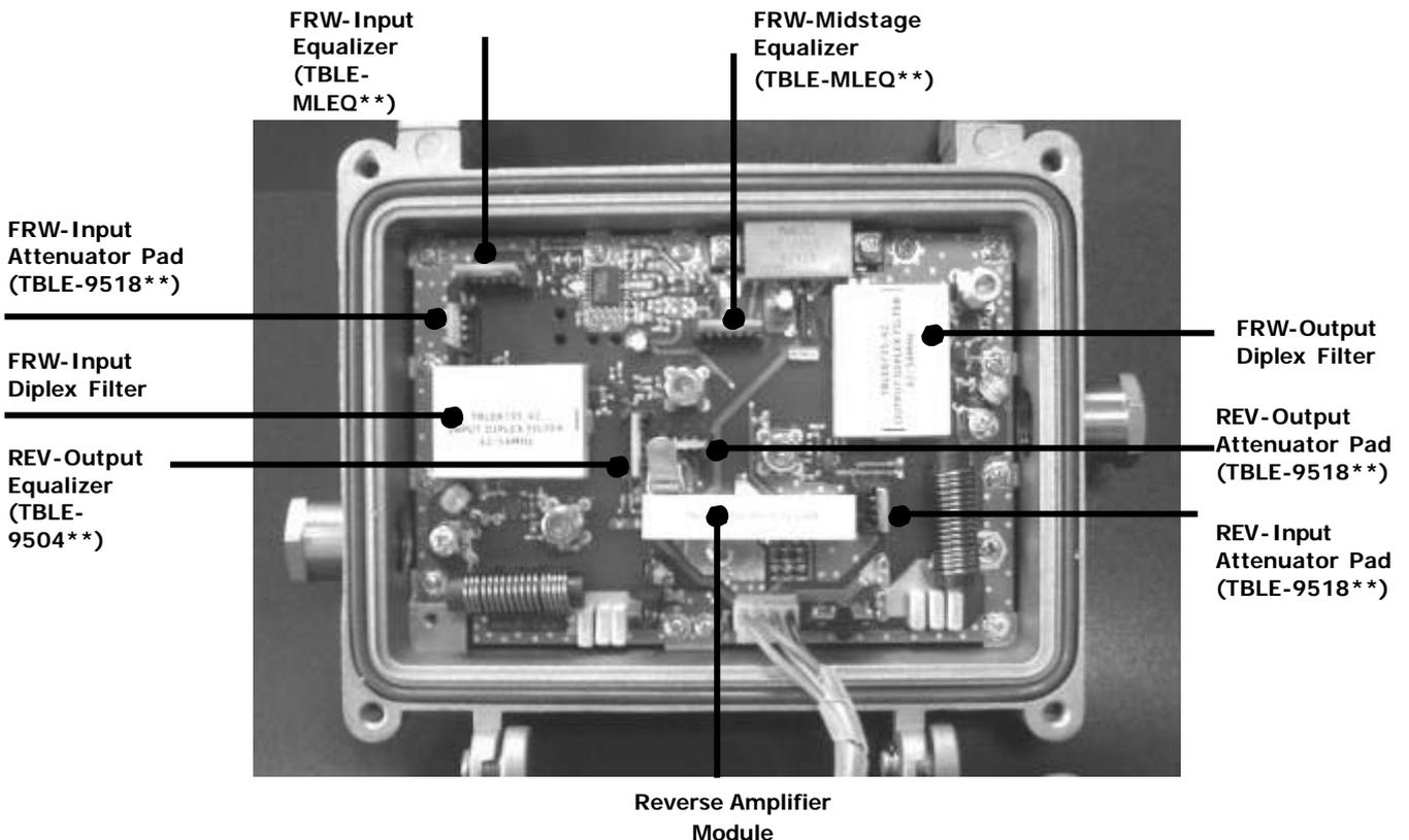
Note: 3 pin sockets are suitable for Attenuator Pads, 5 pin sockets are for Equalizers
