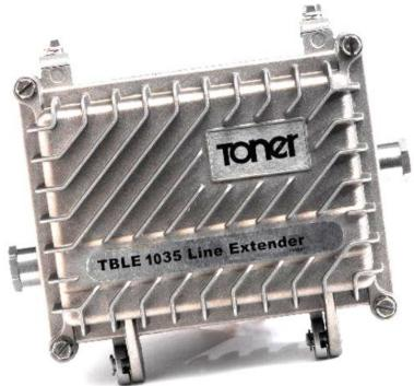
gain reverse amplifier for use in 2 way systems and can be ordered with one of 3 standard sub splits, 42/54 MHz, 55/70 MHz and 65/80 MHz. The diplex filters are the plug in type for easy field changes or repairs.
