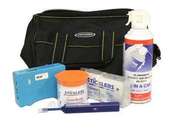
The TFCC contains the equipment needed to clean both the fiber connector end face as well as the bulkhead fitting that they are plugged into. It features a can of air to remove dust from the vicinity of the connection, a bag of sticklers to clean a mating sleeve, clean wipes for cleaning the connectors, a fiber connector cleaner for cleaning the end face of the fiber, a one click bulkhead cleaner for cleaning the fiber bulkhead connection and a handy canvas carrying bag.
