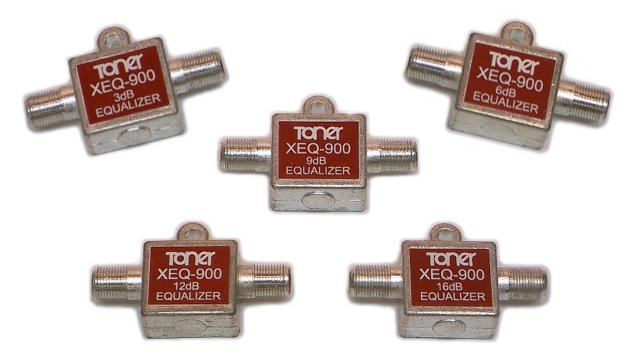
Toner introduces their In Line Equalizers. The XEQ-900-\* equalizers are available in five values: 3, 6, 9, 12, and 16 dB. The XEQ-900-\* will help to compensate for excessive slope in RG cables. Built in a small zinc diecast housing with machined F connectors.
