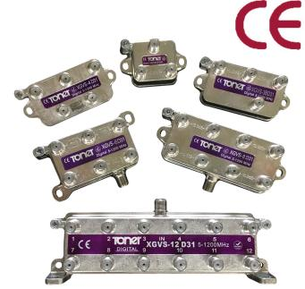
This new series of drop splitters from Toner are designed to work in digital systems deploying DOCSIS 3.1 that utilizes the 5-85 MHz spectrum for upstream, and the 105 to 1220 MHz spectrum for downstream. By using the latest in ferrite core and winding technology along with premium PC boards and components we have been able to increase bandwidth without any sacrifice in performance.
