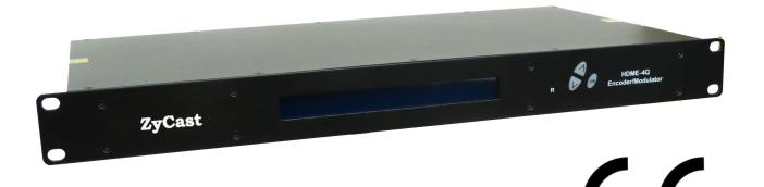
The HDME 4Q is a FOUR program High Definition digital modulator with a 4 channel, 2 QAM output. With the HDME 4Q you can convert video signals into Digital TV channels for distribution to any number of TV's on the system. The HDME was engineered to work with Satellite receivers, Digital Signage players, DVD players, Media players and any other device with a video output.
