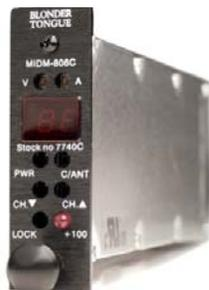
The MIDM is a professional quality agile audio/video demodulator and is intended for both CATV and VHF & UHF analog applications. The unit is in a "single width" Die-Cast housing that allows deployment of up to 12 demodulator units in a MIRC-12 chassis.
