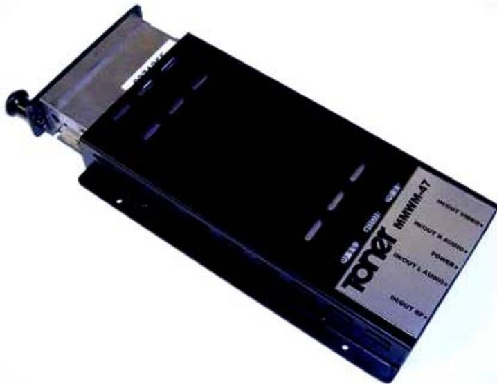
The MMWM-47 is a stand alone chassis designed to hold any of the industries minimod type headend pieces such as a modulator, demodulator, stereo encoder, converter or digital demodulator. The MMWM-47 is ideally suited for wall mounting, using on an A/V cart, or mounting to the back of a TV/monitor. The chassis has four 1/8" diameter mounting holes along the flanges and ventilation slots on the sides for heat dissipation. It comes with a universal power supply for domestic and international use.
