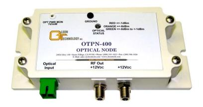
The Olson PremiseNode OTPN-400C Optical Node is a low-cost, compact, indoor CATV receive-only node in a new cast housing. It is designed with the latest optical receiver technology to reliably deliver a full slate of multiplexed video, data, and telephony services in an HFC (hybrid fiber/coax) or PON (passive optical network) broadband CATV environment.
