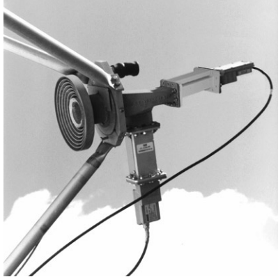
7893D mounted between antenna feed & LNA (both Vertical & Horizontal Polarization)
