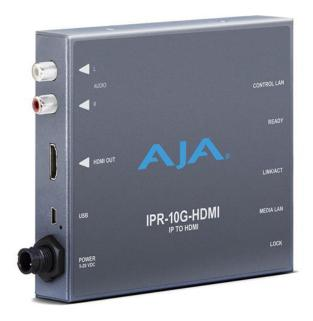
IPR-10G-HDMI provides monitoring of HD SMPTE ST 2110 signals via HDMI. It receives SMPTE ST 2110 over 10 GigE connectivity, formats the data for output on a full-size HDMI interface, and the associated audio from the video stream is extracted, synchronized, and embedded into the HDMI interface and also output on an analog RCA interface.
