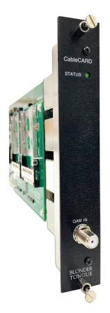
The NXG-CCQD-24 (CableCARD® Input Module) is part of the Blonder Tongue NeXgen Gateway (NXG) platform that decrypts HD and SD programs from a Cable or Telco TV service provider.
