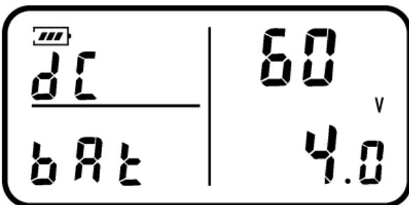
The trunk voltage will show on the higher right and the battery voltage will show on the lower right. AC or DC of the trunk voltage is also indicated on the higher left.
