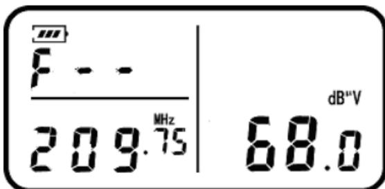
It displays on the higher left “F--”, the lower left is the frequency of the audio carrier; the right is the level of audio carrier (or FM).
