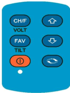
**CH /F** Single Channel/Frequency, Battery Voltage
