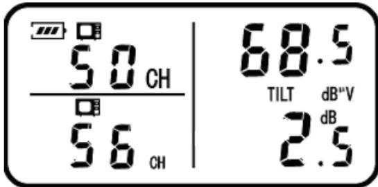
Two channel numbers with max frequency and min frequency among six testing channel are displayed on the left, the higher right is the corresponding level of max frequency channel, the lower right is corresponding Tilt.
