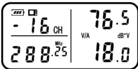
Here the higher left is the measured channel number, the lower left is the video carrier frequency, the higher right is the level of video carrier, the lower right is the  $\Delta V/A$  of the current channel (the level difference between the video carrier and the audio carrier)
