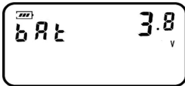
The left displays "BAT " word and the higher right displays the internal battery voltage.
