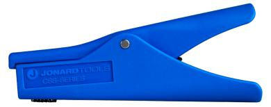
The CSS-59M is a coaxial cable stripper specifically designed to strip the stub end of a mini coax cable in a wall outlet, exposing 9 mm of braid and 7 mm of the center conductor, which eliminates the need to run new cable. This coaxial cable stripper features the following:
