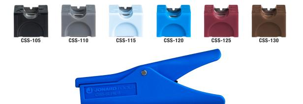
The CSS Series tools are coaxial cable strippers specifically designed to strip a stub end of a coax cable in a wall outlet box, which eliminates the need to run new cable, saving time and money. Each strips RG-59 and RG-6 cables to specific braid and center conductor lengths shown in chart below. The built-in strip stop insures the strip lengths are consistent. VELCRO® strip on bottom of tool is used to fold back braid on cable after being stripped.
