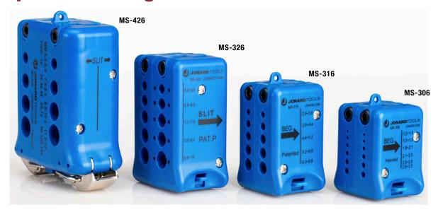
These **PATENTED** slit and ring tools are designed to open fiber jackets and loose buffer tubes to provide easy fiber access. One side of the tool slits fiber jackets and loose buffer tubes, the opposite side rings fiber jackets and loose buffer tubes. All this is done without damage to the fiber. Blades are replaceable. Note: MS-326 is designed for cables used in ducts and microducts.
