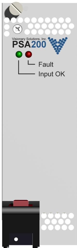
Two LEDs are provided on the PSA200:
