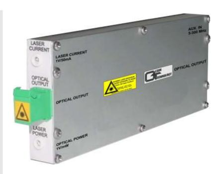
The Olson Technology OTPT-300A is a cost-effective, field-installable return laser transmitter with an RF passband of 5 to 300MHz. The unit comes in several models including a 1310nm DFB laser with 3mW output (+4.8dBm), a 1550nm DFB laser with 2.5mW output (+4.0dBm), or a CWDM laser with a 2.5mW output (+4.0dBm). This transmitter is intended only for indoor applications. This transmitter must be mounted to an Olson OTPN-2000C or OTPN-1000. It will not function as a stand-alone device.
