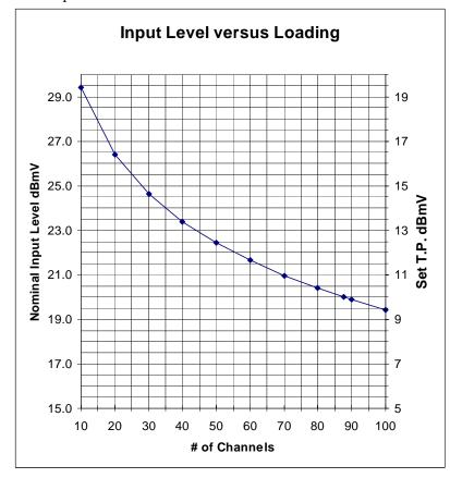
If the channel loading is less than 40, you may decide not to increase the levels by the maximum possible amount. This will provide improved distortion at the cost of S/N. The best rule of thumb is to use the maximum possible levels for long haul links, and lower drive levels as the links get shorter.
