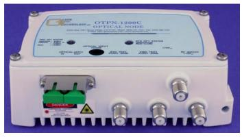
The Olson Technology, Ind. **OTPN-1200C-H/L** *PremiseNode* is a compact, cost-effective, full-featured indoor CATV node designed using the very latest optical receiver technology to reliably deliver a full slate of multiplexed video, high speed data and telephony services in an HFC or PON broadband CATV environment.
