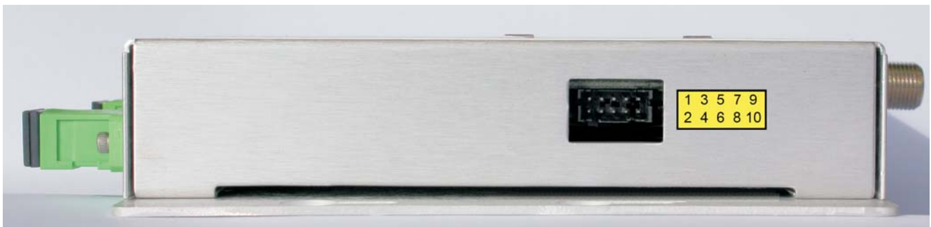
FIGURE 2 - Electrical Connector Pin Configuration
