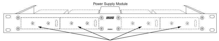
FIGURE 1 - Front Panel View of RMM4. Space allows for up to four mini-modules (modules not included).
