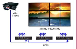
Using cascading feature to implement 4x3 video wall
