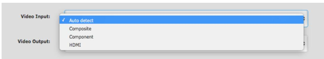
Selecting HDMI, Component, or Composite “locks” the encoder to detect only the input type selected.
