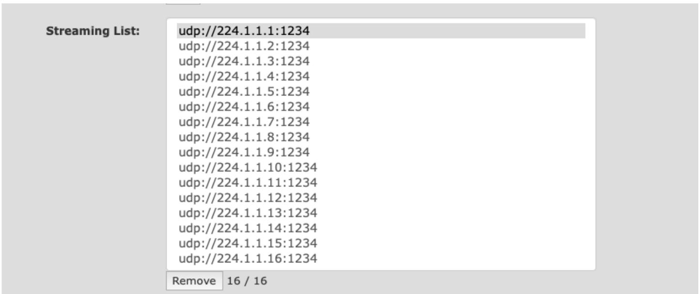
Note: The HDME-I/P-3 can have up to 16 different Multicast Addresses.
