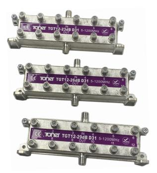
This new series of from Toner are designed to work in digital systems deploying DOCSIS 3.1 that utilizes the 5-85 MHz spectrum for upstream, and the 105 to 1220 MHz spectrum for downstream. By using the latest in ferrite core and winding technology along with premium PC boards and components we have been able to increase bandwidth without any sacrifice in performance.
