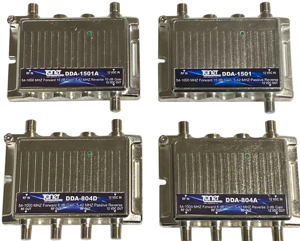
The Toner DDA (Digital Drop Amp) is the newest drop amp model available from Toner. These RF amplifiers feature a precision compact die cast aluminum housing for superior performance and so they can be fitted into the tightest of spaces. Four different amplifier models are available to fit just about any installation requirement. Two with passive reverse (1 and 4 output) and two with active reverse (1 and 4 output). Frequency range is 5 to 42 MHz reverse and 54 to 1000 MHz forward.
