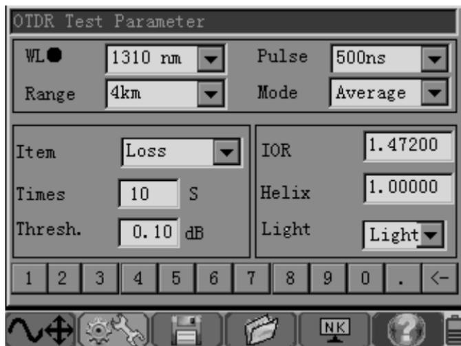
Figure 2-9 OTD-1315 parameter setting interface
