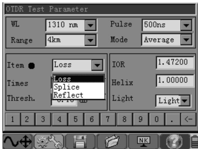
Fig. 2-11 Setting of test methods of OTD-1315A OTDR
