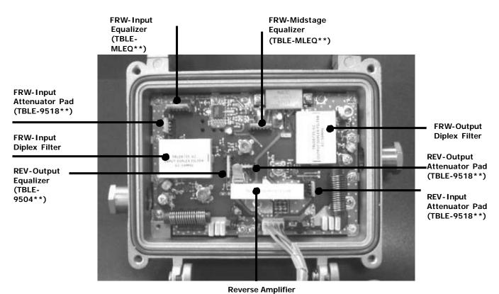
Note: 3 pin sockets are suitable for Attenuator Pads, 5 pin sockets are for Equalizers
