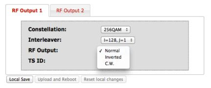
RF Setup tab can be used to modify the Interleaver and RF Output type (if required). Most installations will not require any changes to the default settings.
