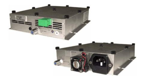
The OLSON TECHNOLOGY INC. LaserLite Model OTOR-300 is a high quality, cost effective CATV Return Path Receiver which utilizes a new low noise, impedance matched, high efficiency 1310/1550nm broadband photodiode and advanced RF amplification circuitry to facilitate carriage of critical downstream video, data, telephony and internet traffic in an HFC broadband environment.
