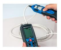
Designed for finding and identifying up to 8 COAX and network cables in main cable boxes, this cable mapper and toner is the perfect tool for use on cables for CATV, network installations, satellite installations, telephone systems, audio-video equipment, CCTV, and security & alarm installations. This 8-way cable mapper and toner kit features the following:
